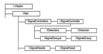
14. Components of traffic signal control within Vissim-COM object model (on the basis of PTV, 2023)
