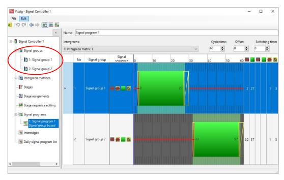
16. Create 'Signal Group' in Vissim GUI with signal plan
